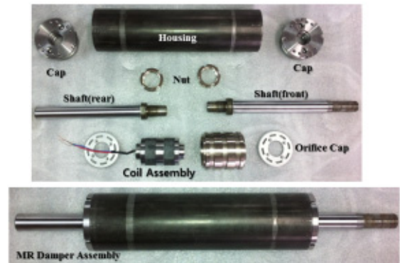
Fig. 6 Photograph of MR damper
