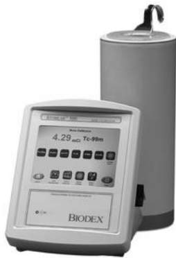
Fig. 4. When using the Dose calibrator, the radioactivity source was set to a volume of 0.1 ml in a 1 cc syringe, placed in a dedicated sample holder, and then radioactivity was measured.
