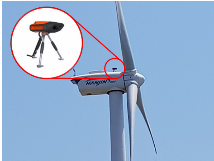
Fig. 3 Nacelle Lidar installed on No. 5 wind turbine of Haengwon wind farm
