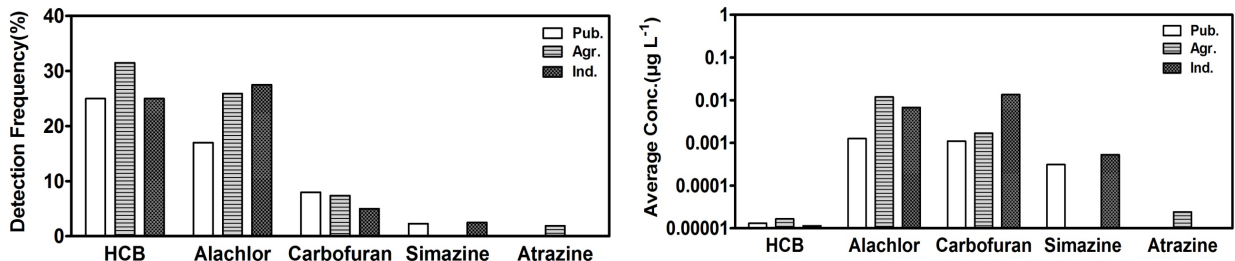
Fig. 8. Detection frequency and average concentrations of pesticides depending on usage of groundwater (Pub.: Public, Agr.: Agriculture, Ind.: Industrial).
