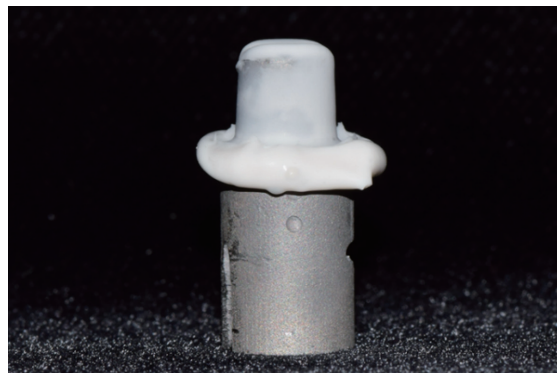
Fig. 2. Silicone replica on metal die.
