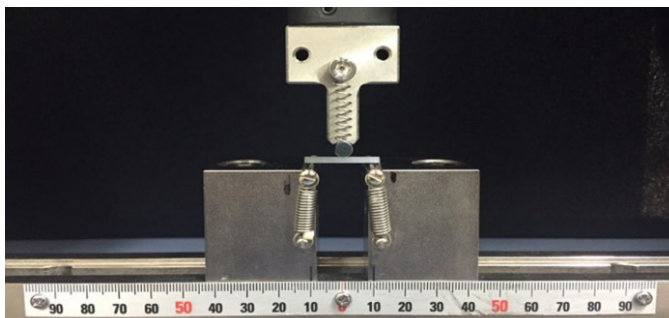
Fig. 1. Three point bending test.
