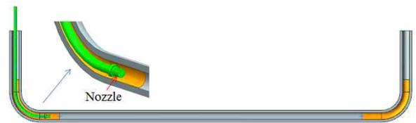
**Fig. 5** Inner shot peening processing section
