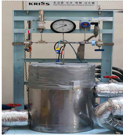
Fig. 2 Hydrogen embrittlement equipment
