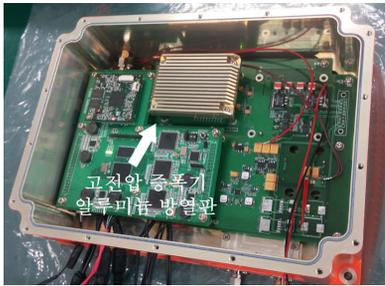
Fig. 4. Aluminum heat sink of HPA
