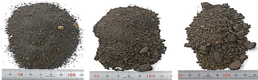
(i) Scrap Ch. & Melting (ii) After 2 nd Ch. & Melting (iii) Flat Bath & Slag foaming
