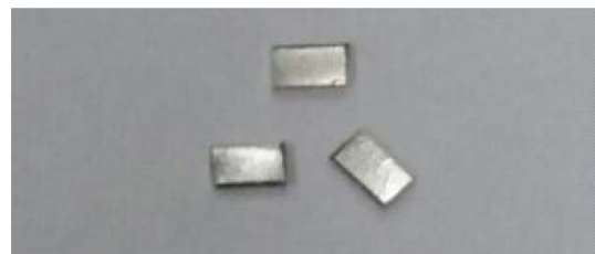
Fig. 7. Thermal fusible parts for thermal fuse system.
