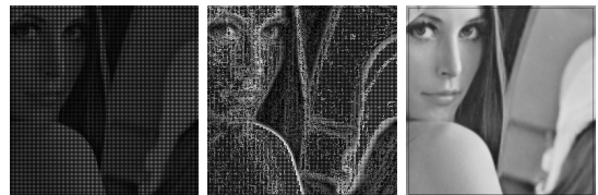
Fig. 6. Step by step results of the proposed interpolation. (a) 1-octave up-sampling (b) H, V, and D directional interpolation (c) Residual pixel interpolation.
