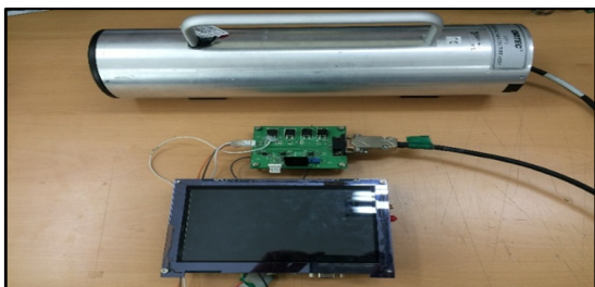
Fig. 3 Analog Portable Radiation Detecting System Structure
