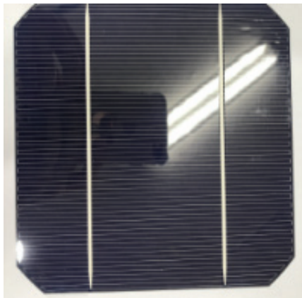
Fig. 4. Si Solar Cell applied wavelength conversion sheet.
