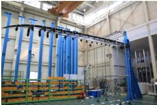
Fig. 14 Wing Static Strength Test Setup
