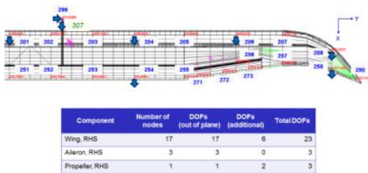
Fig. 19 Accelerometer Locations and Measuring Degree of Freedom for Wing
