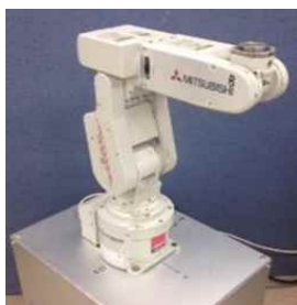
Fig. 3. An industrial 6-axis vertically articulated robot arm
