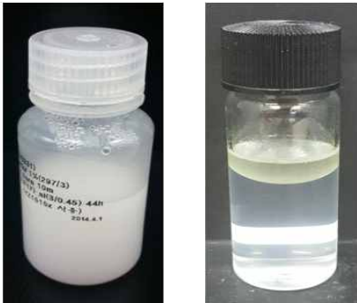
Fig. 4. Image of Emulsion A (left) and Emulsion B (right) after 30 months
