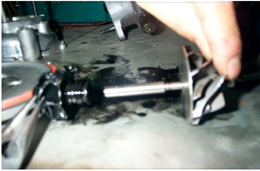
Fig. 5. Turbocharger example by fracture.
