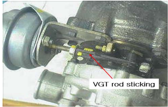
Fig. 6. Sticking example of VGT rod.
