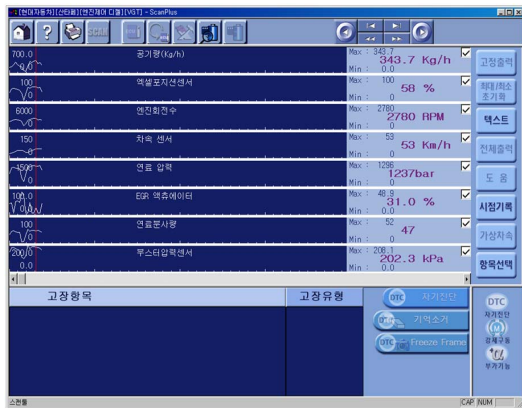
Fig. 8. Measuring datas for troubleshooting after repair.
