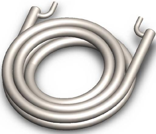
Fig. 6. Shape of outer tube in coaxial heat exchanger.
