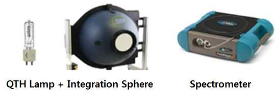
Fig. 2. Image acquisition equipment for radiometric Calibration
