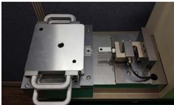
Fig. 7. Photo of load cell, hanger, semiconductor formed plate
