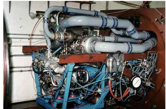
Fig. 3 3-Stage Turbocharger System inside Altitude Test Chamber in TMS [25]
