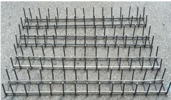
Fig. 2 Photos for main reinforcement and stirrup details
