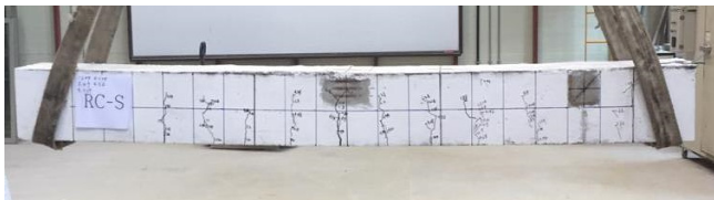
(b) After static loading test
