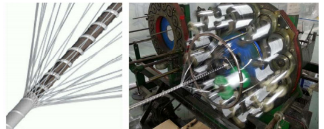
Fig. 4 Manufacturing process of FRPH bar
