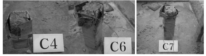
Photo 4 Failure modes of specimen C4, C6, and C7
