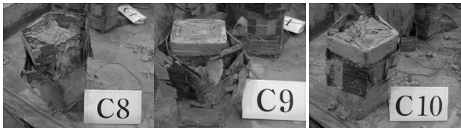
Photo 5 Failure modes of specimen C8, C9, and C10
