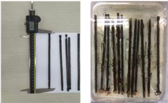
Fig. 3 Photos for rust removal process
