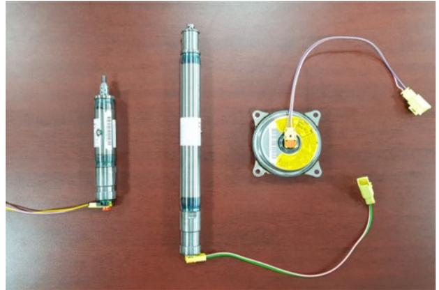
Fig. 1 Side, curtain, driver's airbag inflators (from the left)
