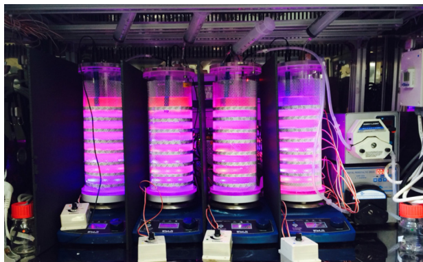
Fig. 1. Experimental microalgae cultivation setup for survey the effects of light irradiation interval.
