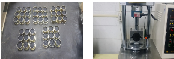
Fig. 2. Marshall stability and flow test
