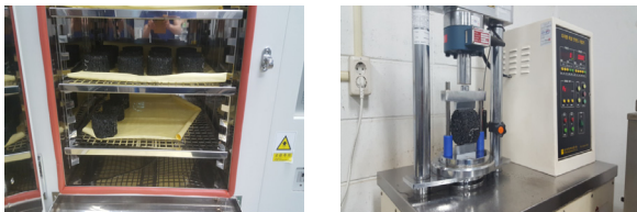
Fig. 3. Indirect tensile strength test and specimen
