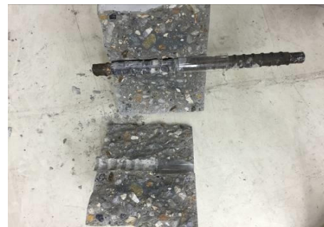
(b) Splitting failure
