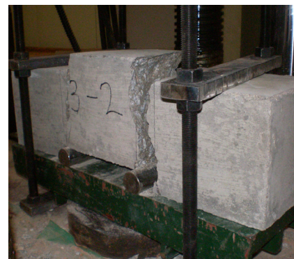
Fig. 4. Photo of test and failure shape
