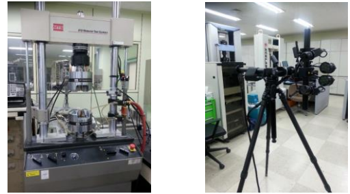
Fig. 2 Schematic view of the equipment for the tensile test
