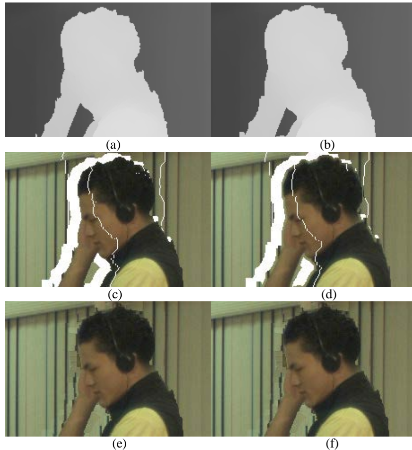
Fig. 9. (a) original depth map; (b) the dilated depth map; (c)3D warping with the original depth map; (d) 3D warping with the dilated depth map; (e) hole filling for (c); (f) hole filling for (d).
