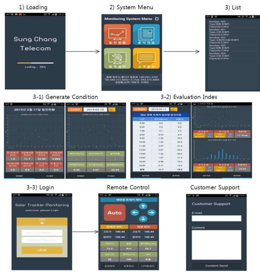
Fig. 8. Notification and remote control using a smart applications
