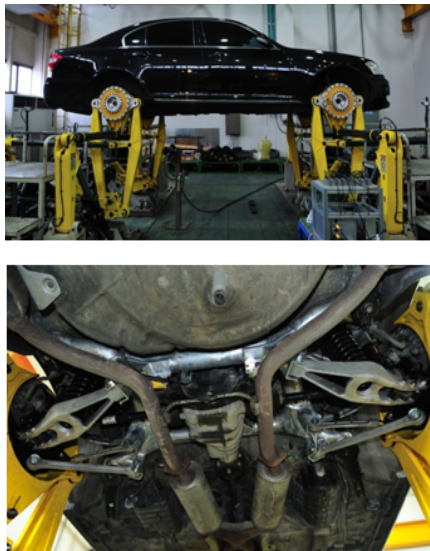
Fig. 7 Road simulator test view of the test vehicle including weight reduction model of torque strut
