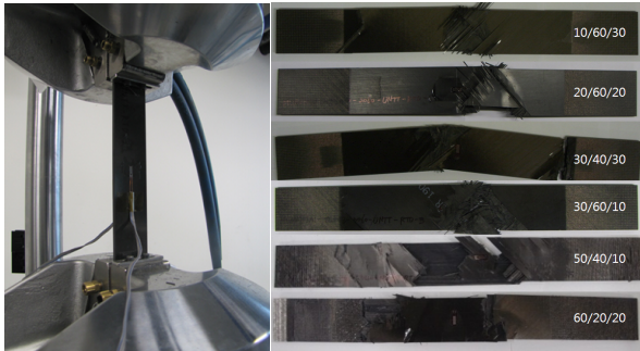
(a) Test set-up (b) Failed tensile specimens
