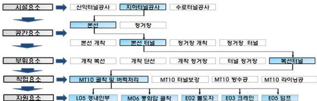
Fig. 4. Subway construction information classification system based on KICT proposal civil information classification system
