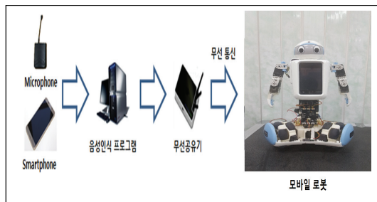
Fig. 15 Remote control schematic diagram of voice recognition robot
