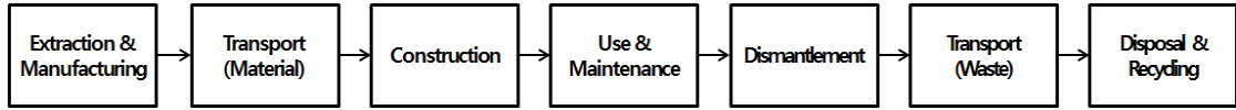
Fig. 3. System boundary of wooden house for the quantification of carbon dioxide emission.
