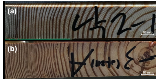
Fig. 6. Wood planks for manufacturing specimens of axial compressive, static bending and shear test. (a) Japanese larch wood plank, (b) Dahurian larch wood plank.
