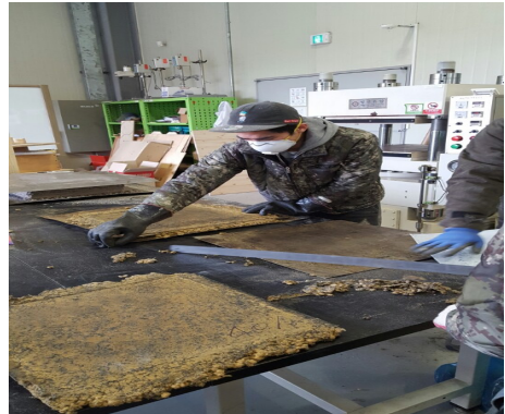
Fig. 1. Manufacturing process on the boards using the carbonized rice husks.
