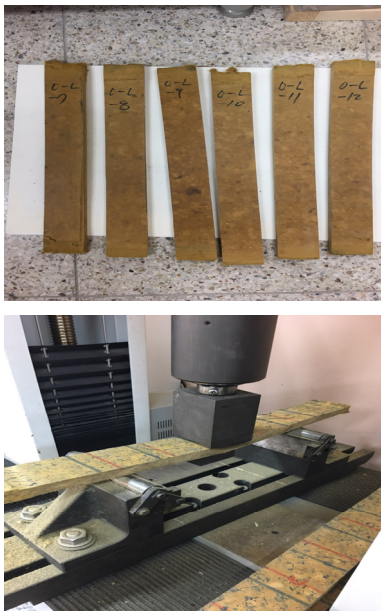
Fig 3. Shape and testing machine for the flexural specimen.
