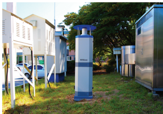
Fig. 1. Ambient gamma energy spectrum measurement device.
