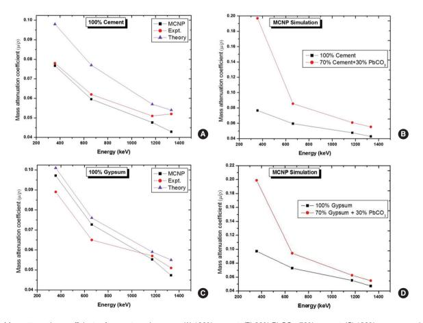
Fig. 2. Mass attenuation coefficients of cements and gypsum. (A) 100% cement, (B) 30% PbCO<sub>3</sub>+70% cement, (C) 100% gypsum, and (D) 30% PbCO<sub>3</sub>+70% gypsum.
