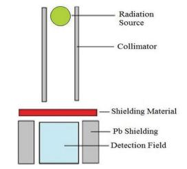
Fig. 1. MCNPX Total simulation geometry for calculations mass attenuation coefficients.
