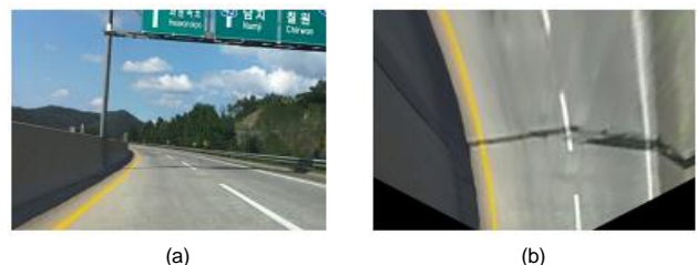
Fig. 1. The effect of image warping. (a) Input image and (b) bird's-eye view.
