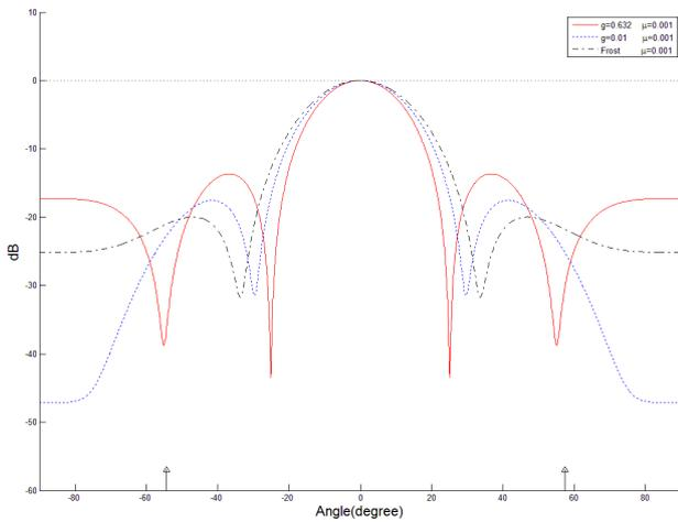
Fig. 5. Comparison of beam patterns for two coherent interference case.
