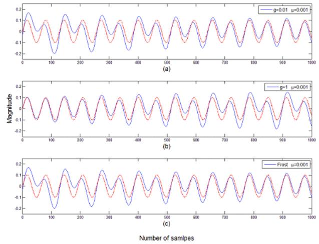
Fig. 7. Comparison of array output and desired signal for one noncoherent interference case for  $1 \leq k \leq 1000$ .
