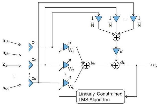
**Fig. 1.** Narrowband general linearly constrained adaptive array.
