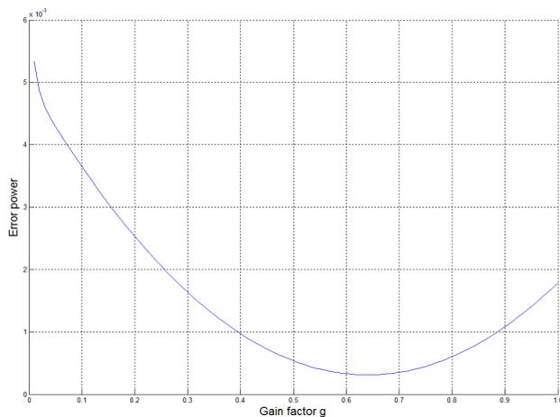
**Fig. 2.** Variation of the error power in terms of gain factor for two coherent interference case.
