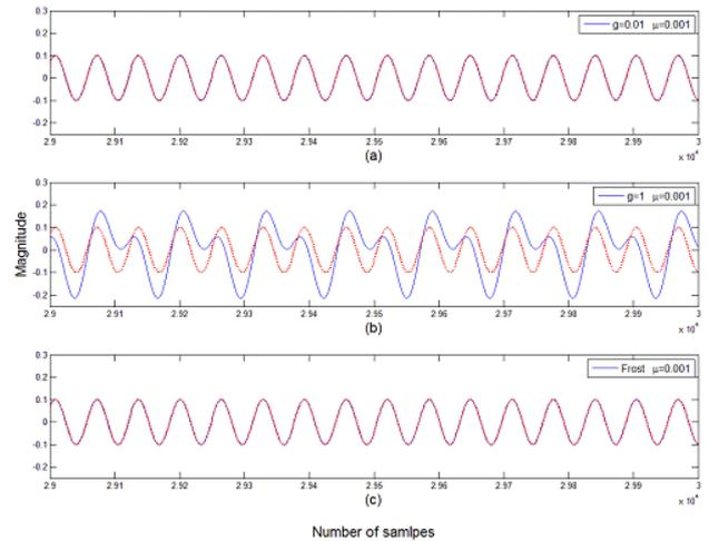
Fig. 8. Comparison of output and desired signal for one noncoherent interference case for  $29001 \leq k \leq 30000$ .
