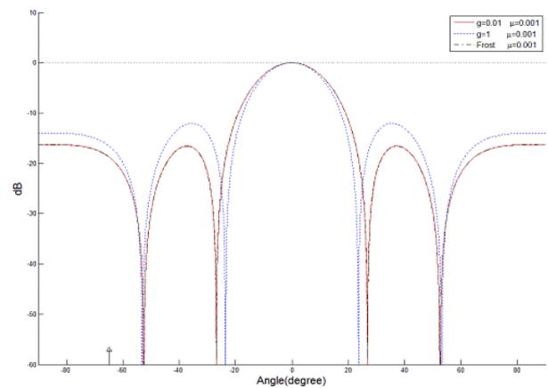
Fig. 9. Comparison of beam patterns for one noncoherent interference case.
