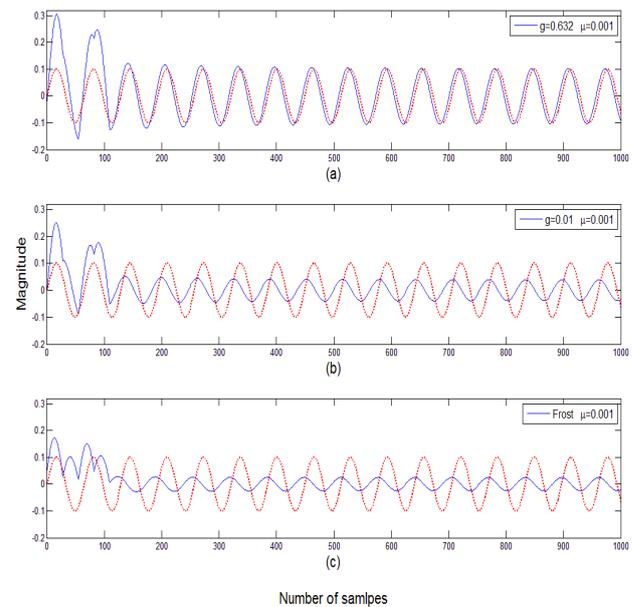
**Fig. 3.** Comparison of array output and desired signal for two coherent interference case for  $1 \leq k \leq 1000$ .
