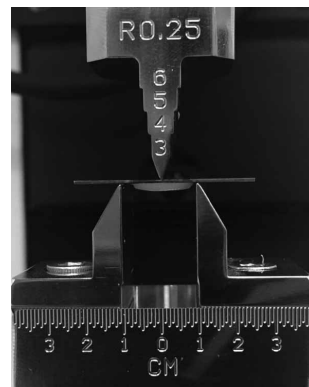
Figure 2. Evaluation of bonding strength using instron model.
