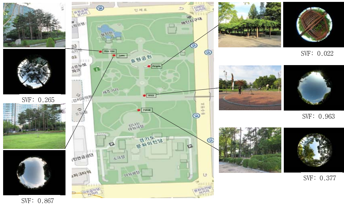
Fig. 2. Five locations in the park (the center map from http://map.daum.net ). Fisheye lens photographs were taken using Nikon Coolpix 8800 camera with Nikon FC-E9 Fisheye converter lens and Nikon UR-E18 converter adapter, and Sky View Factors (SVF) of the photographs were calculated with BMSky-view (Gál et al., 2007).
