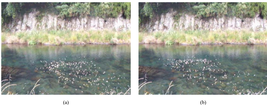
Fig. 6. The direction of movement of the tracking particle and the direction of movement of the water surface; a) 1 sec image, b) 15 sec image.
