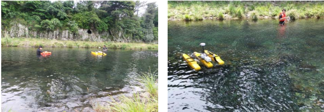
Fig. 3. Site application of ADCP for discharge observation.
