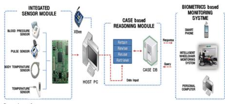
Fig. 3. Configuration of system.
