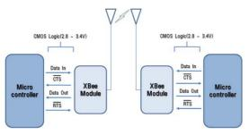
Fig. 4. Configuration of XBee Module Communication.
