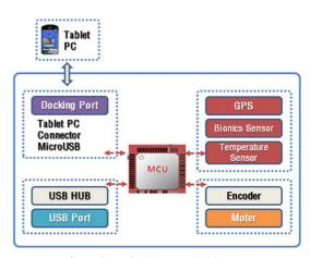
Fig. 6. Configuration of tablet PC docking system.
