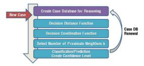
Fig. 2. k-NN Algorithm execute process.
