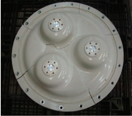
Fig. 9. The cracked insulation barrier by performing internal pressure test.
