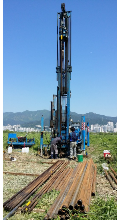
Fig. 3. Modified standard penetration test (SPT) employed to sample aquifer sediment in the Nakdong River Delta. The method is basically the same as conventional SPT except modified split barrel sampler.
